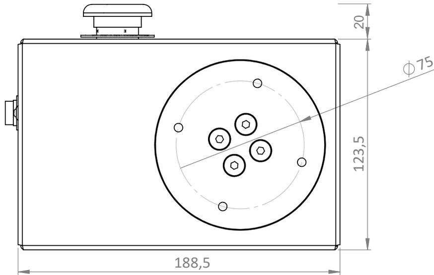
**Figure 4: Dimensions - Top View**
