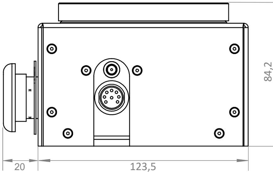
**Figure 3: Dimensions - Front View**
